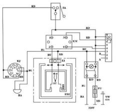
Ko: Power switch KM: AC contactor HA: Buzzer X1: Terminal FU: Fuse (25A SA: Sensitive switch CH1 C
